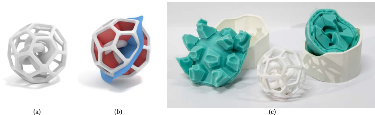
Fig. 1. Our technique for casting extremely complex shapes up to (a) objects made up of multiple entangled pieces. (b) We design a cut layout in the mold volume, which is defined by a parting surface membrane (blue) and a set of additional membranes to enforce moldability (red). (c) We assemble a composite mold made up of a hard plastic shell and a soft silicone part, and then fabricate the given object using liquid casting techniques.
