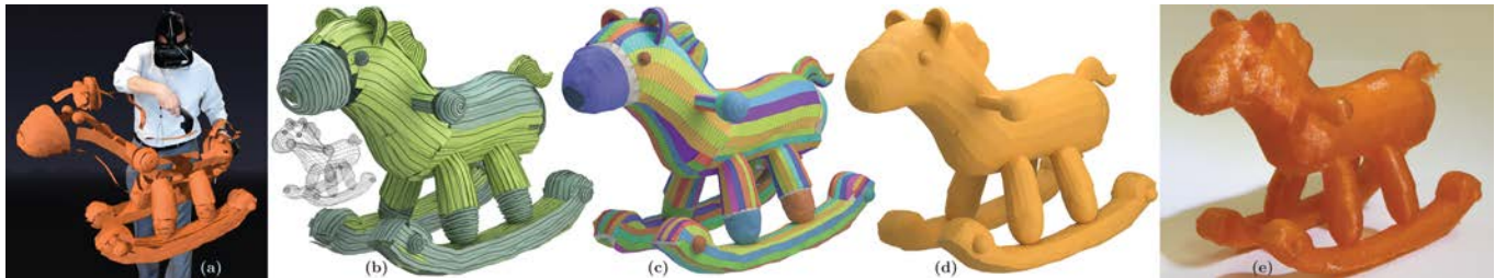
Fig. 1. (a) Drawing 3D strokes using a VR brush. (b) Completed 3D brush-stroke drawing with central stroke polylines drawn in black and ribbon color reflecting normal orientation (green for front, turquoise for back, inset shows polylines alone). (c) triangle mesh strips connecting adjacent stroke polylines (multicolor), and gray triangle strips that complete the surface connecting differently directed stroke groups. (d) Final output. (e) Fabricated model. Input drawing: © Jafet Rodriguez.
