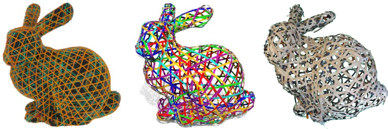
Fig. 1. We present new algorithms for computing geodesic foliations on discrete surfaces. A geodesic foliation on a six-fold branched cover of the Stanford bunny (left) describes the ribbon layout of a triaxial weave (center), which we fabricate out of birch veneer (right).
