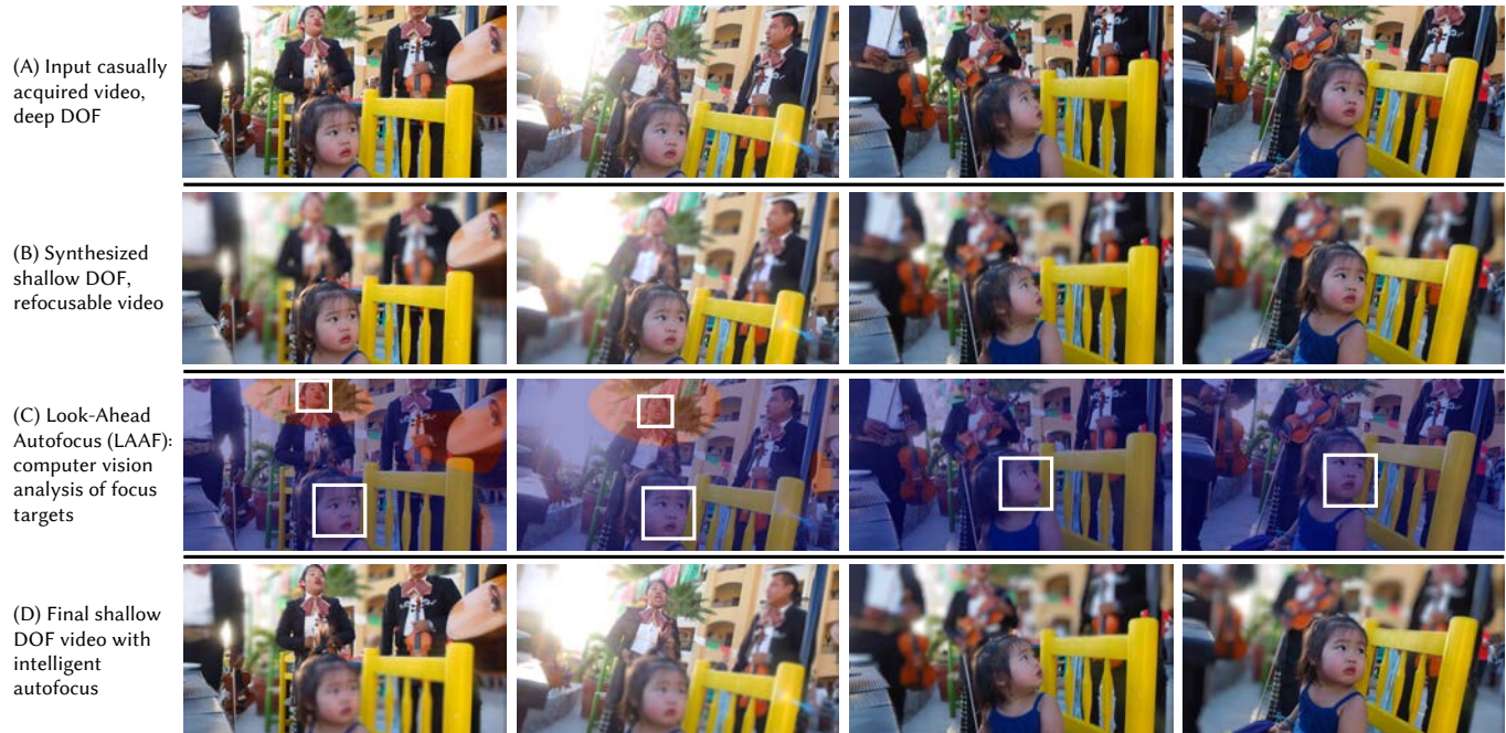
Fig. 1. We present a new approach to pursue cinema-like focus in casual videography, with shallow depth of field (DOF) and accurate focus that isolates the subject. We start with (A) a deep DOF video shot with a small lens aperture. We use a new combination of machine learning, physically-based rendering, and temporal filtering to synthesize (B) a shallow DOF, refocusable video. We also present a novel Look-Ahead Autofocus (LAAF) framework that uses computer vision to (C) analyze upcoming video frames for focus targets. Here, for example, we see face detection (white boxes) and localization of who is speaking/singing [Owens and Efros 2018] (heat map). The result is shallow DOF video (D), where LAAF tracks focus on the singer to start, and transitions focus to the child as the camera pans away from the musicians. The LAAF framework makes future-aware decisions to drive focus tracking and transitions at each frame. This presents a new framework to solve the fundamental realtime limitations of camera-based video autofocus systems.
