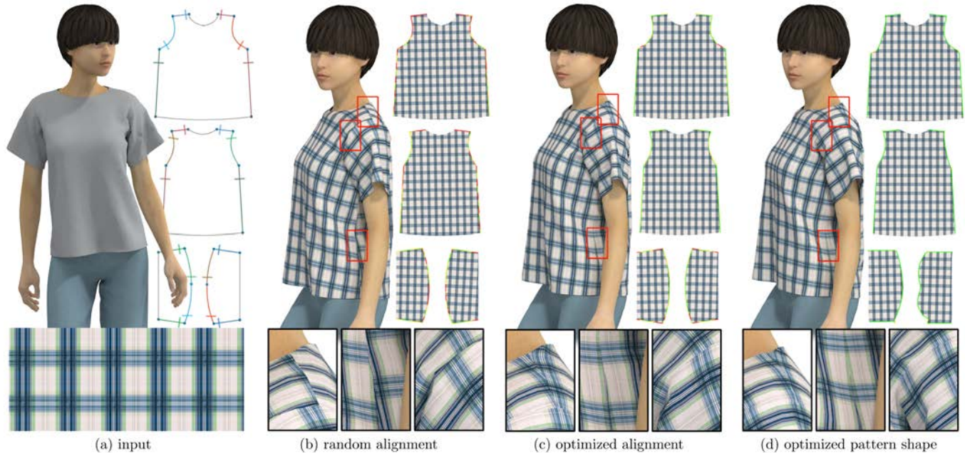
Fig. 1. Our method supports the production of high quality textured garment designs by optimizing the continuity and symmetry properties of the texture across seams. Our input is a sewing pattern and the desired fabric texture, or a 2D wallpaper pattern (a). A random placement of the sewing pattern on the fabric is likely to result in obvious misalignment of the texture on the seams, which is visually displeasing (b). Our method computes an optimal placement, such that misalignments of the repetitive wallpaper pattern are minimized (c). For most garment shapes, it is impossible to achieve a perfectly seamless appearance without changing the shape of the sewing pattern itself. Therefore we additionally provide the option to slightly alter the sewing pattern shape to obtain a much better texture fit along the seams (d). The improved visual appearance is noticeable in the 3D simulation of the garment, while the shape remains close to the original design. See also Fig. 3. The mismatch at each seam edge is visualized on a color scale from green (0 cm) to red (2 cm).
