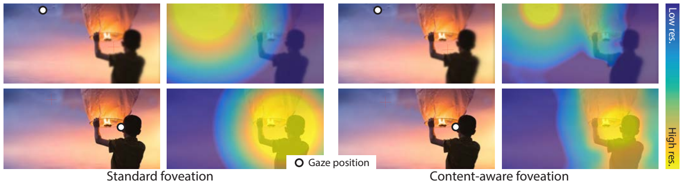
Fig. 1. Current foveated rendering techniques (left) use a fixed quality decay for peripheral vision. While this can be a conservative solution, it does not provide a full computational benefit. Our technique (right) performs content-adaptive foveation and relaxes the quality requirements for content for which the sensitivity of the human visual system at large eccentricities degrades faster. Image by pixel2013 / Pixabay.
