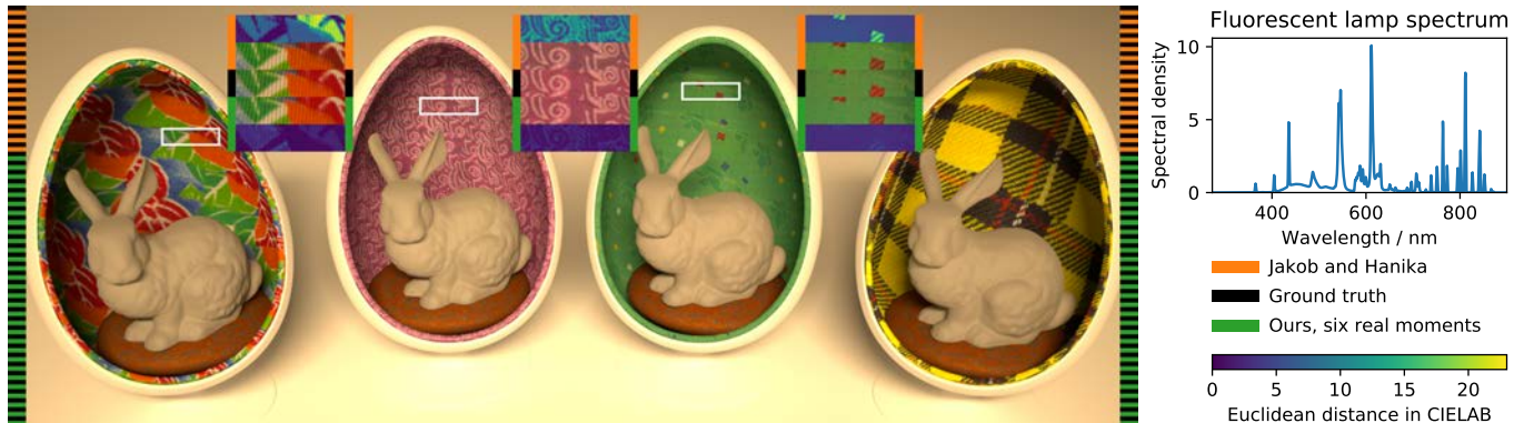
Fig. 1. We store six moments per texel in 8 bytes to represent the spectral albedo textures in this scene. Our novel reconstruction method (green stripes) uses this data to approximate the actual reflectance spectrum. Thus, color reproduction is accurate, even with challenging illuminants such as the fluorescent lamp used here. The interleaving in the upper part, the magnified insets and the insets with distances in CIELAB show how strongly state of the art tristimulus techniques [Jakob and Hanika, 2019] (orange stripes) deviate from ground truth (black stripes).
